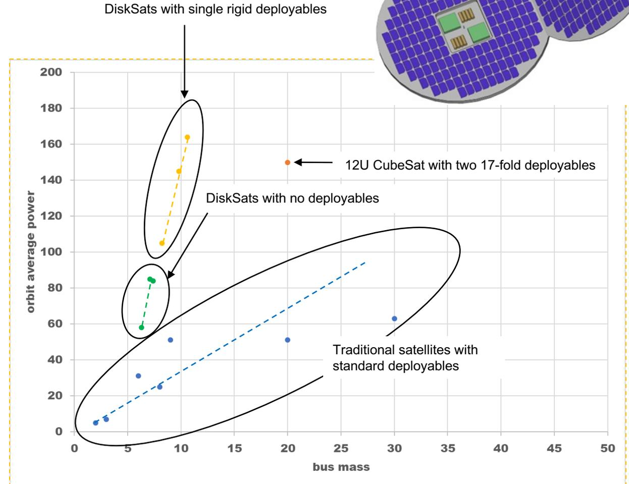
Typical orbit-average power available from various satellite bus designs assuming comparable LEO orbits
