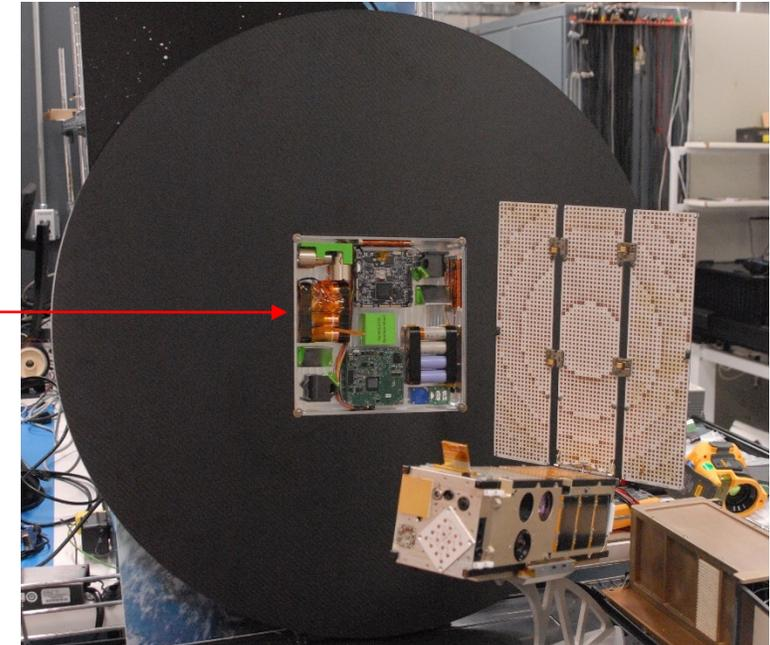
***The DiskSat is an efficient approach to building and deploying constellations of very small satellites***
