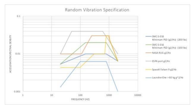
**Figure B.3.4.** Enveloped random vibration environment at interface to spacecraft.
