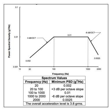
Figure 4.1. - Minimum vibration spectrum.
