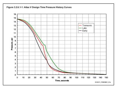
Figure 3.6. Typical Pressure decay curve<sup>7</sup>. (Courtesy of ULA)
