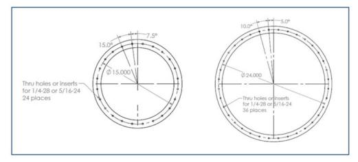
Figure 3.8. Standard 15" & 24" port interface bolt patterns<sup>9.</sup>
