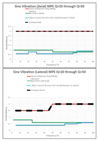
Figure 3.4. Potential sine vibration environment for several launch vehicles and spacecraft general specification.
