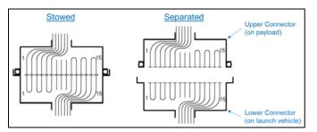
Figure 3.12. Separation loop back signals.
