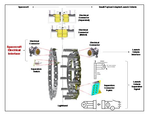
Figure 3.11. Spacecraft electrical interface to separation system.
