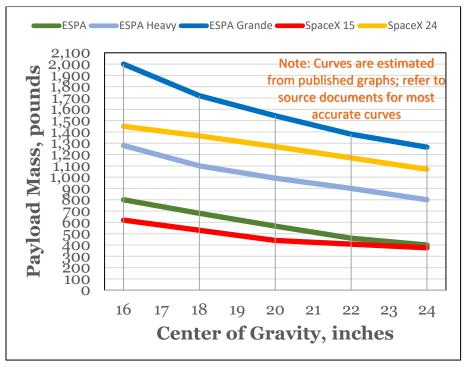
Figure 3.10. Mass – Center of Gravity Curve 6 & 9.
