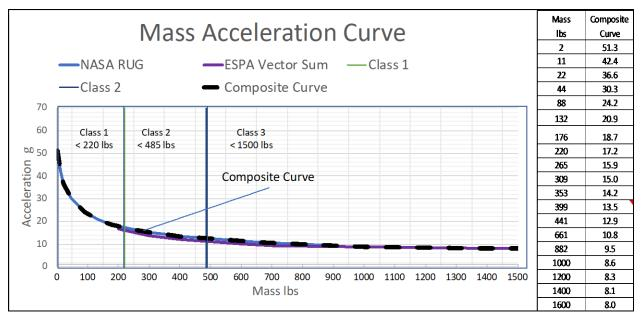
Figure 3.1. Mass acceleration curve for spacecraft quasi-static loading.
