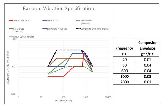
Figure 3.2. MMDS enveloped Random Vibration Requirements.
