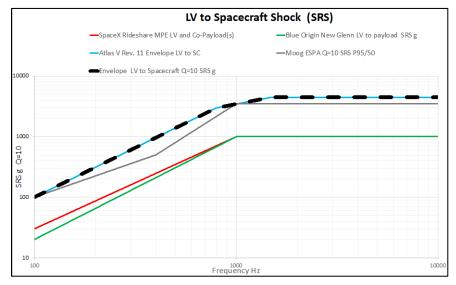
Figure 3.5. Maximum predicted launch vehicle and co-payload SRS and maximum allowable SRS produced by the spacecraft.
