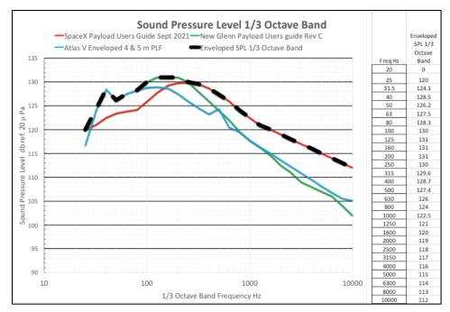
Figure 3.3. Enveloped Sound Pressure Levels within the fairing in dB.
